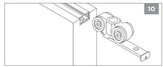
Position leading roller in the hole furthest from edge of door.
