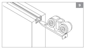
Position rear roller in the hole closest to the edge of door.
